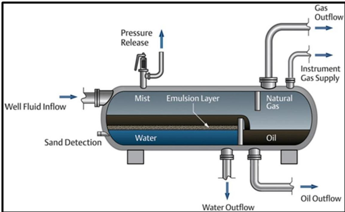
Figure 12: Schematic of Test Separator (Emerson website, 2017).
