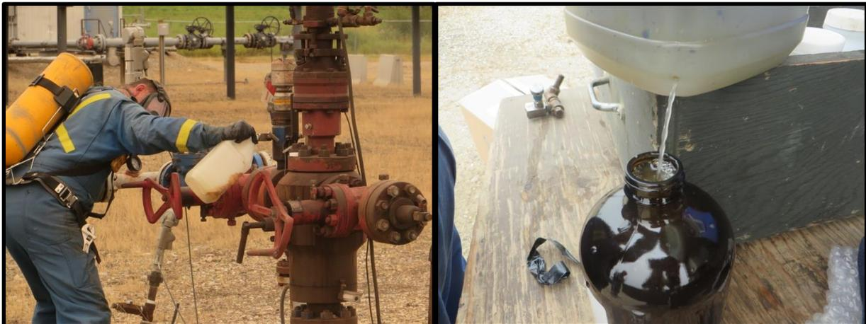
**Figure 11: Sample collection at wellhead. Left: Maxxam employee sampling from access port into 4 L plastic container. Right: Decanting brine sample from bottom of 4 L container.**
