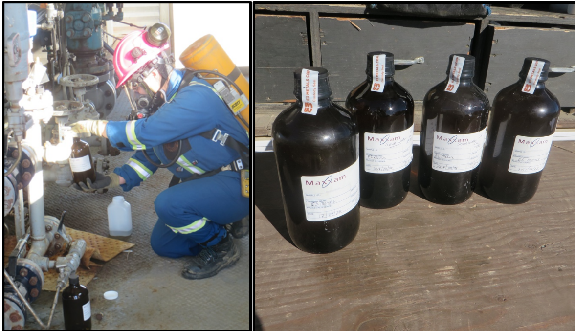
Figure 13: Sample collection at test separator. Left: Maxxam employee collecting sample from test separator access port. Right: Sealed well samples.
